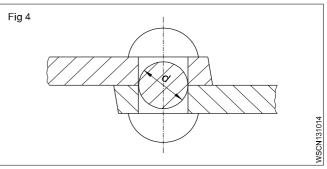
Rivet cross-section is the hole cross-section.
